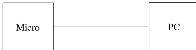
The same arguments apply to Example 2 where we are talking to a PC but be warned that the micro may be easily overwhelmed by a flood of UDP messages pumped out by a 1700 MHz PC. If large amounts of data are to be exchanged or the application structure suits it we might use FTP, the File Transfer Protocol, which is an optional MicroNet module.
